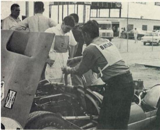
“SCIENTISTS connect magnetic tape recorders to a racing car at Daytona during a series of experiments to determine physical stress of driving in competition. Test results may aid astronauts in space flights. News Photo by Chuck Rogers.”
