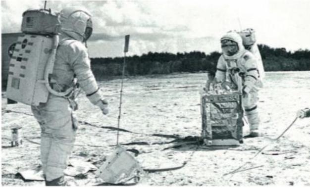
"APOLLO 14 backup Commander Eugene Cernan, right, and backup Lunar Module Pilot Joe Engle go through lunar surface exercises at KSC. Engle, deploying box-like four-barrel devices which will be left behind to hurl explosive charges at ranges up to 5,000 feet while Cernan is at the central recording and relay station which will transmit the seismic data back to Earth."
