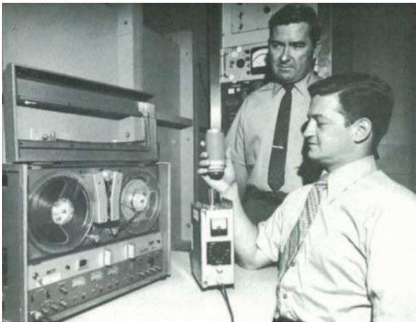
"DAVID R. INGALLS, right, Supervisor of the Acoustic Calibration Laboratory at KSC's Central Instrumentation Facility, conducts a pre-launch test of recording instruments that are used by Information Systems' Measurement Systems Division to measure decibel or noise levels resulting from the blastoff of Saturn V launch vehicles. Wilson R. Timmons, Chief of the Test Analysis Section, observes the results of the test."
