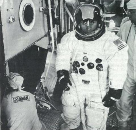
“APOLLO 16 Commander John Young enters the lunar module in an altitude chamber in the MSO Building where he and Lunar Module pilot Charles Duke successfully completed a verification run with the chamber pumped down to a simulated altitude of more than 200,000 feet. Command Module Pilot Thomas Mattingly will participate with Young and Duke in the command-service module altitude run.”
