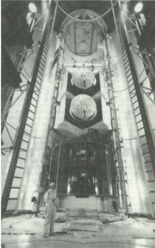
“A RECORD three-satellite payload was hauled into space by Orbiter Discovery during the new spacecraft's maiden flight. Major cargo components visible in this photo of the cargo bay prior to launch, are, at top (or front), the Office of Aeronautics and Space Technology-1 (OAST -1) experiment; and, in descending order, the Satellite Business Systems-D, TELSTAR 3-C, and the LEASAT-2 (SYNCOM IV) satellites.”
