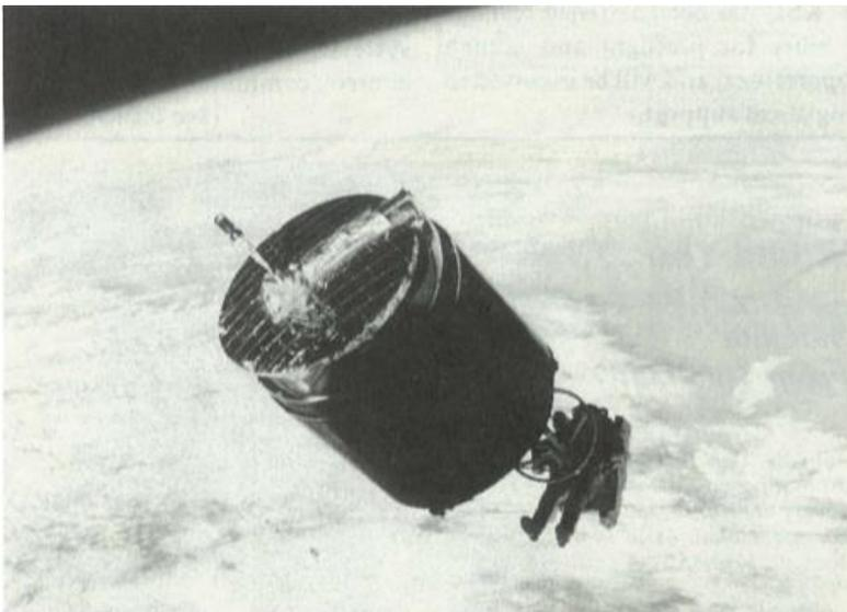
"ASTRONAUT GARDNER captures the orbiting Westar by inserting the stinger device into the spacecraft's aft section>
