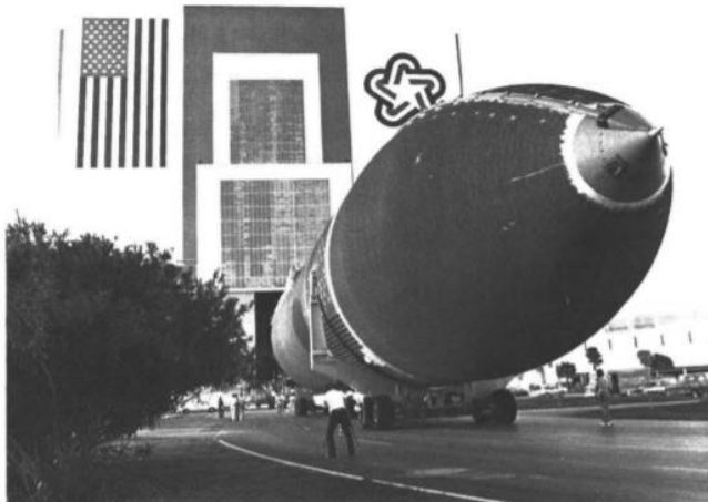
“TANKING UP- The external tank scheduled to fuel the STS-27 launch of Atlantis is moved into a storage cell at the Vehicle Assembly Building March 30. Workers began preparing ET-23 for flight last week.”
