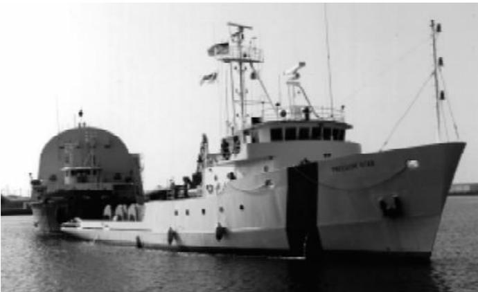
"Freedom Star, one of NASA's two solid rocket booster recovery ships, towed a barge
