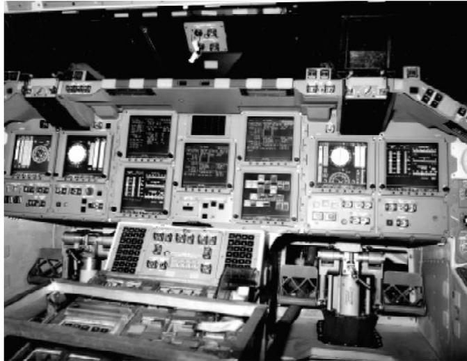
“The first fully digital cockpit for Shuttles is now in Atlantis. Full-color displays replace buttons, knobs and dials. Photo credit: Tom Tschida, NASA Dryden Flight Research Center.”
