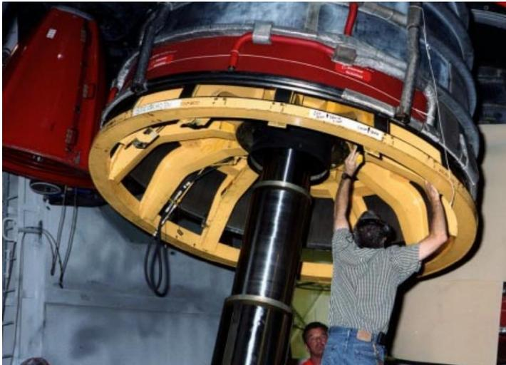
“Workers in the Vehicle Assembly Building oversee the replacement of Main Engine No. 1 in Space Shuttle Atlantis. Because of concerns about a possibly defective fuel pump tip seals, launch managers decided to replace the engine with one scheduled for installation on Discovery. The main engine nozzle, visible in the photo, is 7.8 feet across and 9.4 feet high...”.
