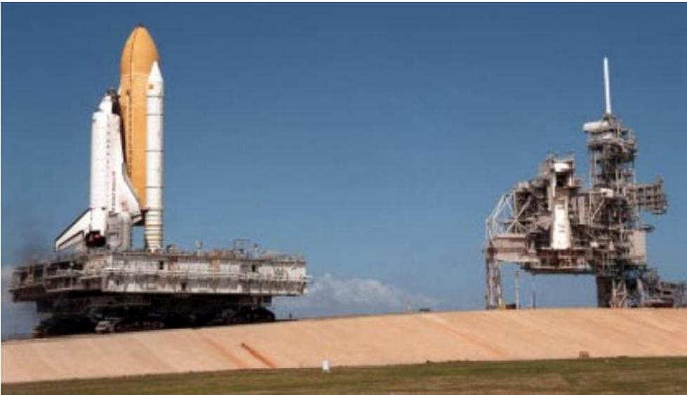
“The Space Shuttle Atlantis, riding aboard the Mobile Launcher Platform, ascends the ramp to Launch Pad 39A on March 25. The platform, which travels at about 1 mile per hour while carrying an orbiter, tilts to keep the flight assembly in a level position during the climb to the pad. Atlantis will carry a crew of seven on STS-101, a mission dedicated to the maintenance of the International Space Station....”.
