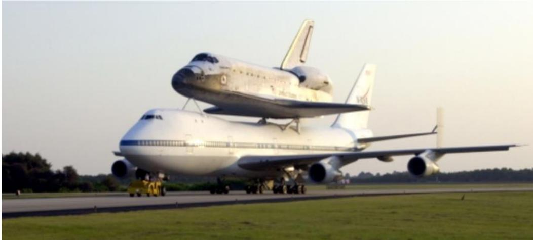
“The Shuttle Carrier Aircraft, with Discovery attached to its back... on the runway at Kennedy Space Center’s Shuttle Landing Facility on Nov. 3. The SCA returned Discovery to KSC after the orbiter’s California landing at Edwards Air Force Base at the end of mission STS-92. Discovery was demated from the SCA via the mate/demate device at the SLF and transported to the Orbiter Processing Facility bay 1 where it is undergoing preparations for its next launch, STS-102, scheduled for February 2001.”
