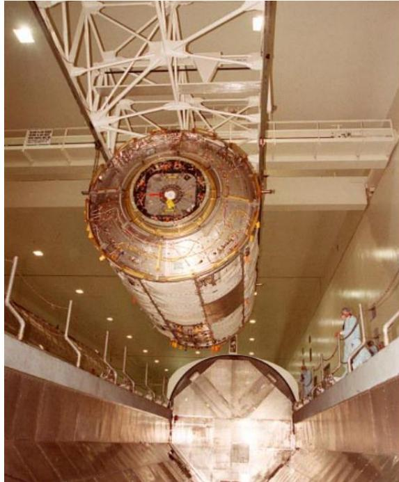
“The U.S. Laboratory Destiny in the Space Station Processing Facility, at left, was rotated before being lifted and lowered, above, into a payload canister. Destiny was transferred to the Operations and Checkout Building for vacuum chamber testing and was determined to be leak free and safe. The module is among more than 216,000 pounds of Space Station elements, including truss sections, that are being prepared for flight at KSC...”.
