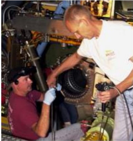
“Gerry Kathka (right), with United Space Alliance, hands part of a fiber-optic camera system to Scott Minnick, who wears a special viewing apparatus for inspecting Endeavour’s flow liner.”
