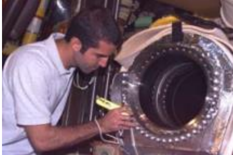
“David Strait, Shuttle systems inspector with United Space Alliance, inspects a Space Shuttle Main Engine flow liner.”
