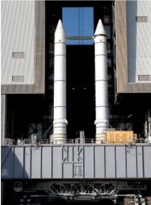
“AS THE CRAWLER TRANSPORTER slowly moves the Mobile Launcher Platform (MLP) out of the Vehicle Assembly Building, the two solid rocket boosters on top are framed in the doorway. The move is in support of engineering analysis vibration tests on the crawler and MLP.”
