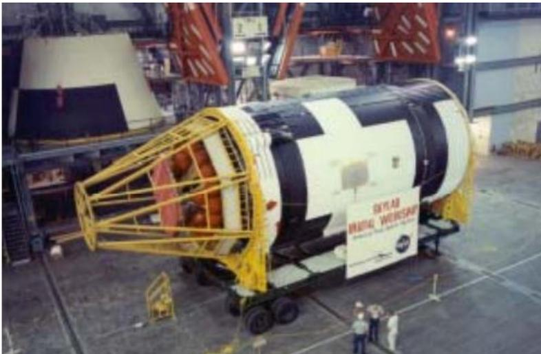
“Skylab was an orbiting space station comprising the Orbital Workshop, Airlock Module, Apollo Telescope Mount and Multiple Docking Adapter.”
