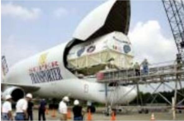
"Node 2, the pressurized module of the Japanese Experimental Module (JEM) is offloaded at the SLF."
