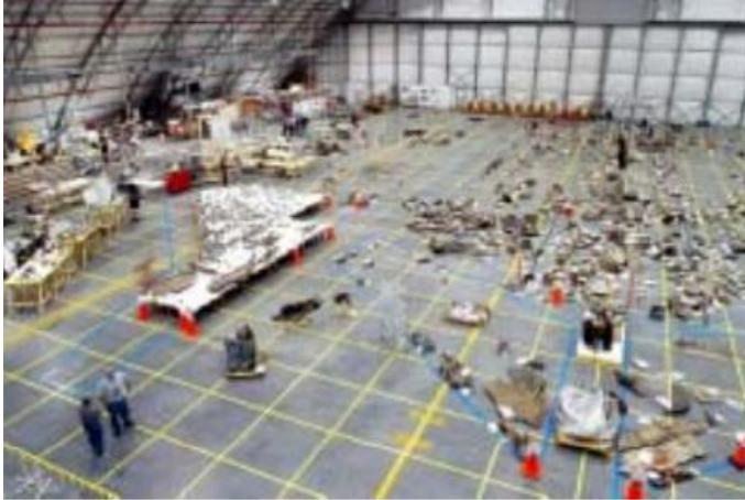
This is a view of Columbia's reconstructed remains in the Space Florida hangar at the Shuttle Landing Facility.
