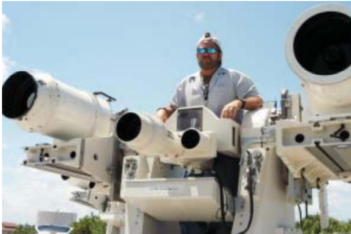
"NASA camera operator Kenny Allen stands in the center console area of one of the recently acquired Contraves-Goerz Kineto Tracking Mounts (KTM)."
