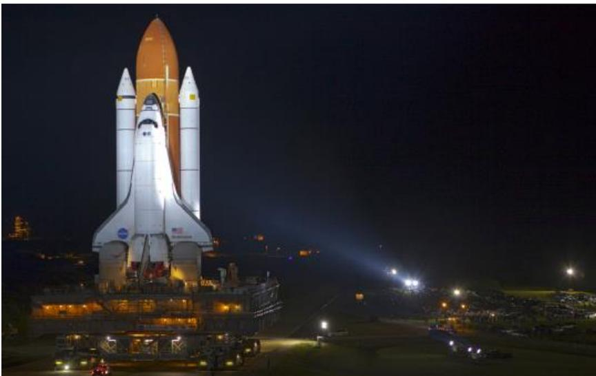
"Bathed in xenon lights, space shuttle Endeavour makes its nighttime journey from the Vehicle Assembly Building to Launch Pad 39A at Kennedy Space Center on March 10. Riding atop a crawler-transporter attached to its external fuel tank and solid rocket boosters, Endeavour's 3.4-mile trek, known as "rollout," began at 7:56 p.m. EST. This is the final scheduled rollout for Endeavour."
