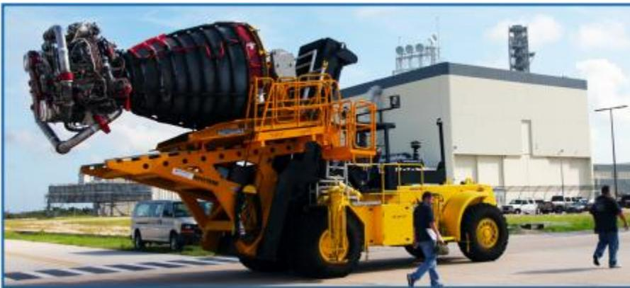
“Technicians transport Engine No. 1, the final engine removed from space shuttle Atlantis, to the Engine Shop for possible future use Aug. 22...”.
