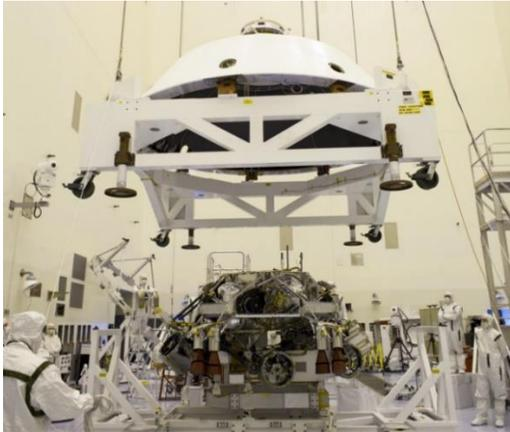
“In the Payload Hazardous Servicing Facility at NASA’s Kennedy Space Center in Florida, technicians guide the backshell as it is lowered over NASA’s Mars Science Laboratory (MSL) rover, Curiosity, for encapsulation on Sept. 23. The backshell, a protective cover, carries the parachute and several components used during later stages of entry, descent and landing...”.
