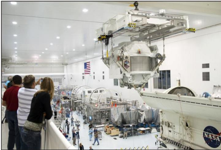
"The Alpha Magnetic Spectrometer-2 (AMS) is moved March 15 from the weight and center of gravity stand, where final measurements were taken before launch, to a payload canister in the Space Station Processing Facility at Kennedy Space Center. The canister will protect the space-bound payload on its journey to Launch Pad 39A, where it will later be installed into space shuttle Endeavour's payload bay..."
