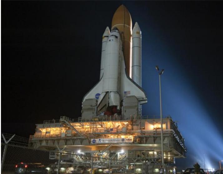
“Xenon lights illuminate space shuttle Discovery as it makes its nighttime trek, known as “rollout,” from the Vehicle Assembly Building to Launch Pad 39A at Kennedy Space Center on Jan. 31.”
