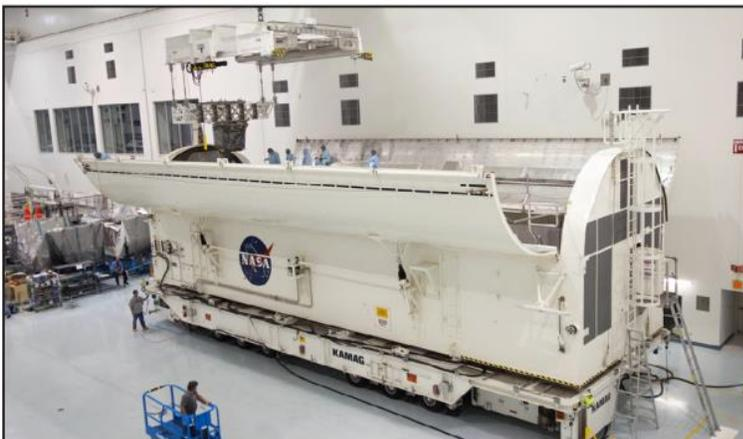
"An overhead crane lowers the Lightweight Multi-Purpose Experiment Support Structure Carrier, or LMC, into a payload canister in the Space Station Processing Facility on May 23. The canister then will be installed into Atlantis' payload bay for the STS-135 mission to the International Space Station. STS-135, the final mission of the Space Shuttle Program, is targeted to launch July 8..."
