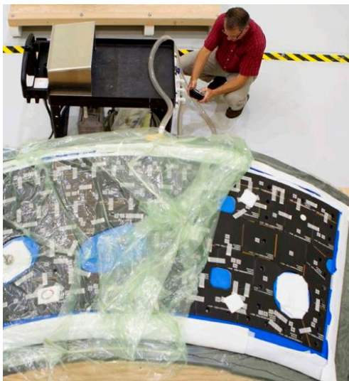
"Technicians have begun bonding thermal protection system tiles to the nine panels that will cover the Orion crew module for the agency's first uncrewed flight test with the Space Launch System (SLS)... in the Neil Armstrong Operations and Checkout Building at Kennedy Space Center."
