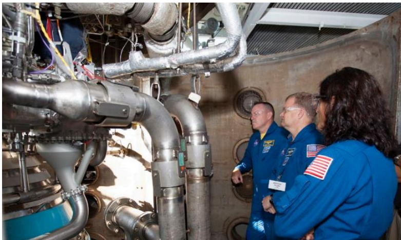
“NASA astronauts Barry “Butch” Wilmore, from left, Eric Boe and Suni Williams survey an RL10 engine as it stands in a vacuum chamber at Aerojet Rocketdyne’s test stand in West Palm Beach, Florida.”
